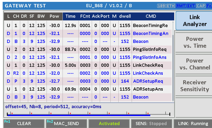
Fig 3.30 Example of communication with Class B Gateway
