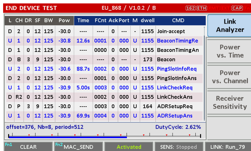
Fig 3.17 MAC command transmission through PING slot
